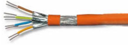
CAT7 1000 MHz S/FTP (S-STP) Kablo 4 x 2 x AWG23/1 PIMF, FRNC-B, 100 Ohm
