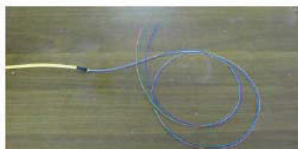
Pic4: fiber after stripping
