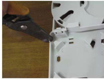
Pic7: right-routing leads in box entrance
