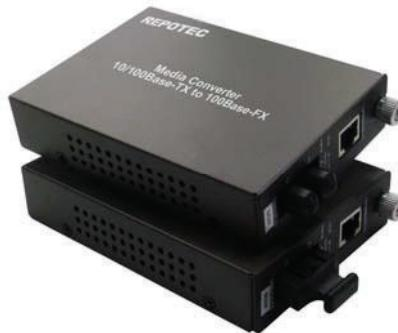
IEEE 802.3/u Ethernet supports two types of media for network connection such as 10/100Base-TX and 100 Base-FX. The bridge media converter is designed with a switch controller and buffer memory that connects two types of segments to operate smoothly. This converter can be used as a standalone unit or as a slide-in module to the 19" converter rack(up to 16 units) for use at a central wiring closet.
