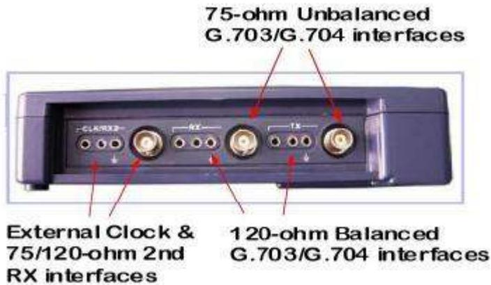
TM101A 2Mbit/s Digital Transmission Analyzer integrates many advantages of several kinds of imported 2M meters. The final design has passed the inspection of communication measurement center, which belongs to information industry.
